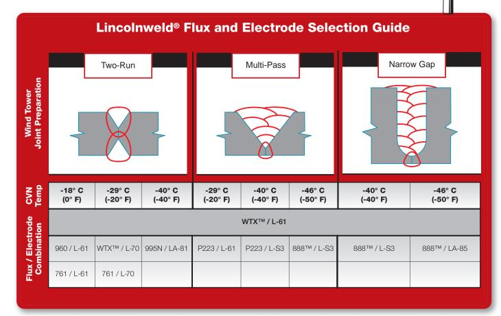
NOTE: Base material dilution is typically 60 - 70% in Two-Run applications, so the Charpy V-Notch (CVN) values will vary significantly with changes in the base metal chemical composition.
