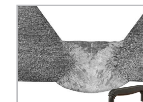
Open gap root pass welded with STT® technology
