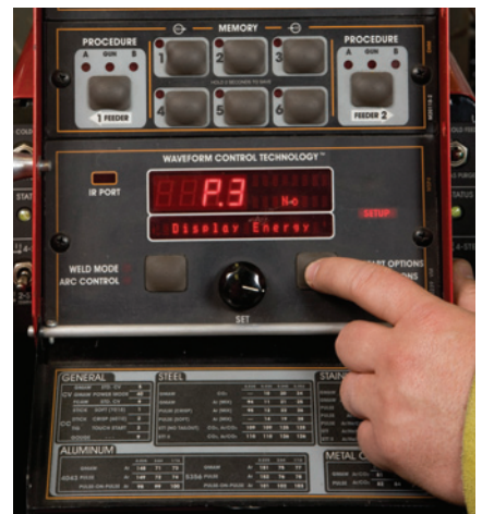
Fig. 2 — With the proper software installed, access to the energy reading entails pressing the menu option "Display Energy."
