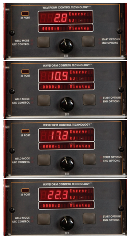
Fig. 3 — The real-time energy is continuously incremented while welding, and the final energy is displayed until the next arc start.
