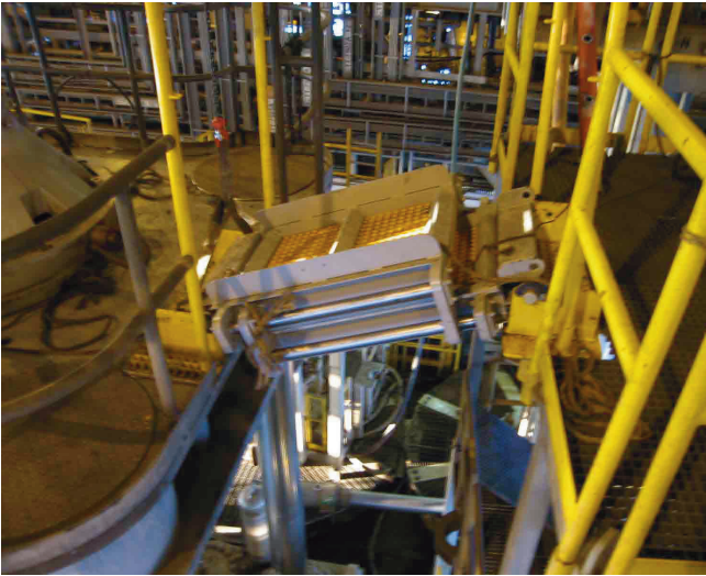
Figure 5. Duron Systems has patented a articulating walk-over structure that allows crews to safely gain access to platforms to perform routine inspections of trees and their associated equipment.
