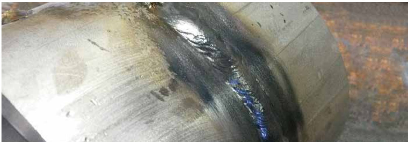
Stable arc and regular welds in PF(up) / 5G Up position
